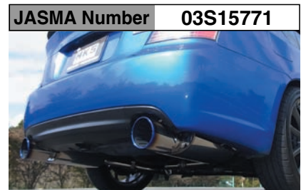
備考 Main + Mid pipe. Compatible with factory rear bumper skirt and/or exhaust finisher installed vehicles.
