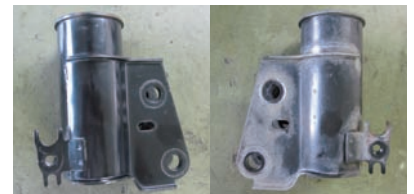
PNE Coating (Left) Common galvanization (Right) * Drove 18,000km in snow area.
